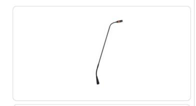
57cm long condenser microphone suitable for placement on lecterns in churches or conference rooms. It has a 3-pin XLR connector and a light curtain that indicates the power status. The capsule is capacitor type and requires +48V phantom power. It can be used as a spare part for DMC 973.
