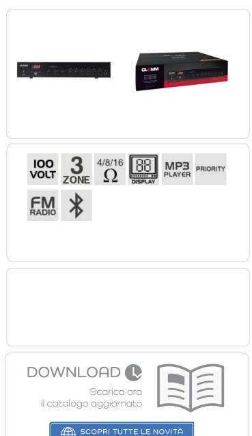
Amplifier operating both at low impedance (4-16 Ohm) and at constant voltage (100V). Its total power of 240W can be either used at will on the 3 zones or be available in the 8-16 Ohm output. The zones are endowed with independent volume. It features 2 mic inputs (the first one with priority function), 1 line input and 1 line output. The built-in MP3 player can play songs from USB sticks and has its own independent volume. It also includes a Bluetooth receiver.
