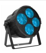
This led spot, made entirely of metal and with control panel on the back panel, features 4 x 60W RGBW COB leds. The beam angle is  $36^\circ$ , with dimmer function and the possibility of controlling all the settings also by connecting it to a DMX 512 system. Thanks to the double bracket it can be mounted on stands or placed on any surface. It can operate both in auto and sound-activated mode, thanks to the built-in microphone. A practical display on the back shows the main functions.
