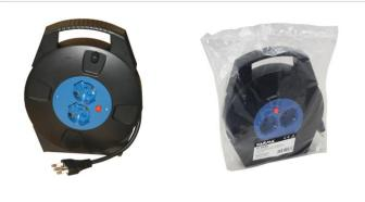
Can be used both at home and for work, it has a 16A plug mounted on an 8 meter retractable cable. Two 10/16A Bipass + Schuko sockets allow you to power two electrical appliances with a maximum load of 1200W (coiled cable) or 3000W (flat cable). A button trips when overloads occur, excluding the voltage supplied.
