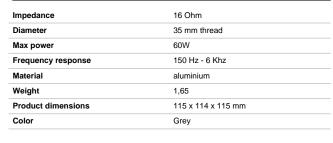
Driver unit for horn speakers with 3,5 cm screw thread. Thanks to the high power and the quality of its materials it offers a very good performance.
