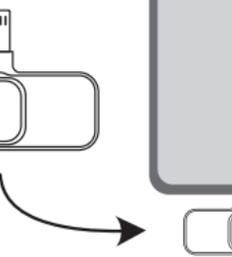
If you wish to recharge the smartphone while using the wireless microphone, you can connect your lightning cable to the side USB socket.
